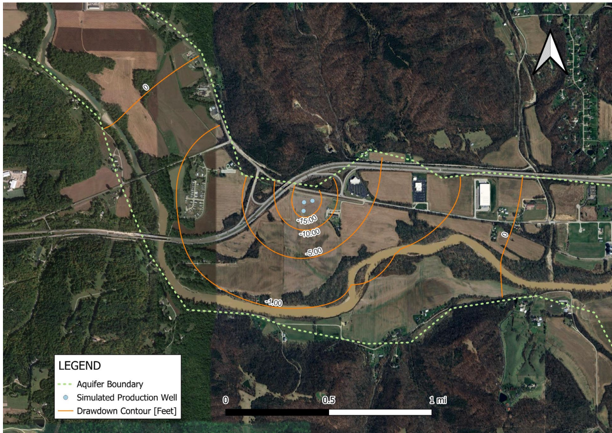
Figure 8. Simulated drawdown resulting from pumping three production wells at the project site for a combined total of 2 MGD.
